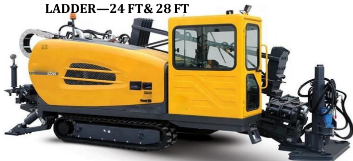
HORIZONTAL DIRECTIONAL DRILLING (HDD) MACHINE
